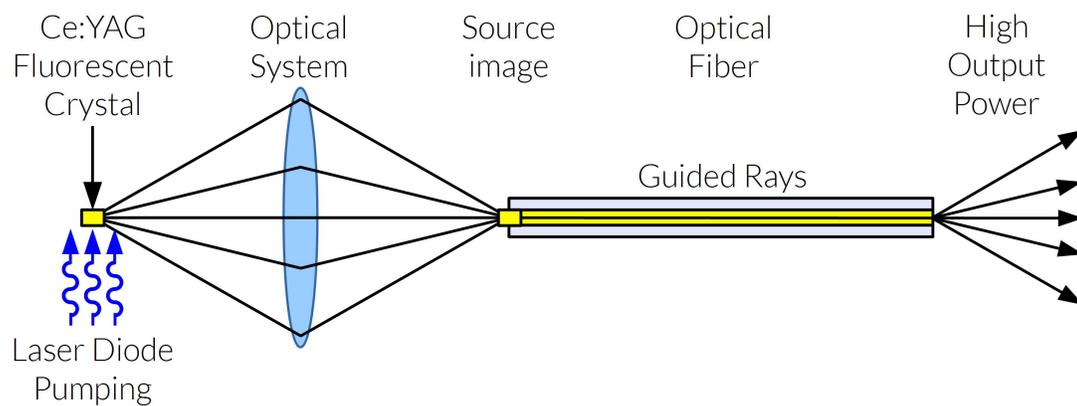
*Laser diode pumped Doric Ce:YAG Fiber Light Source*
