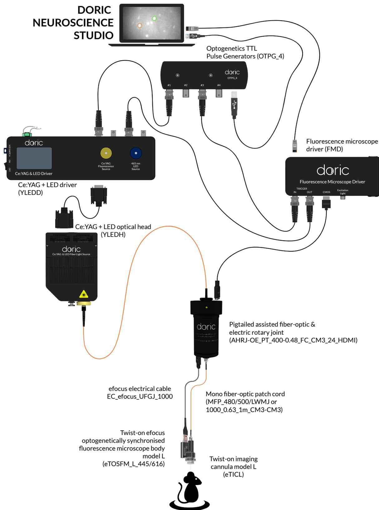
*Twist-on efocus Optogenetically Synchronised Fluorescence Microscopy System for Deep-brain Imaging of GCaMP6*
