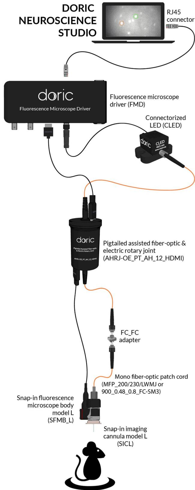
Basic Fluorescence Microscopy System for Deep-brain Imaging of GCaMP6
