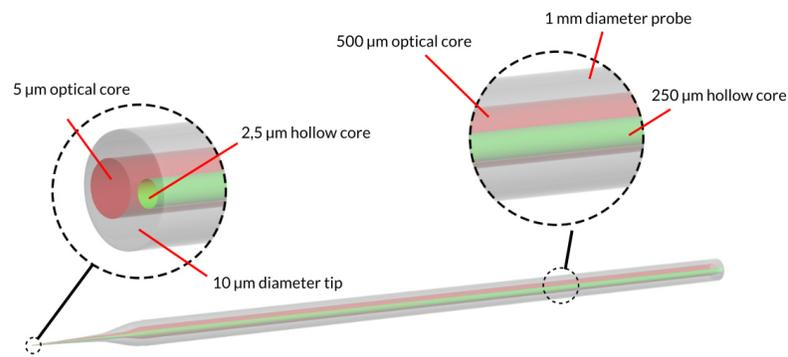
Single-cell Recording Opto-electric Probe Tip of 10  $\mu\text{m}$  diameter
