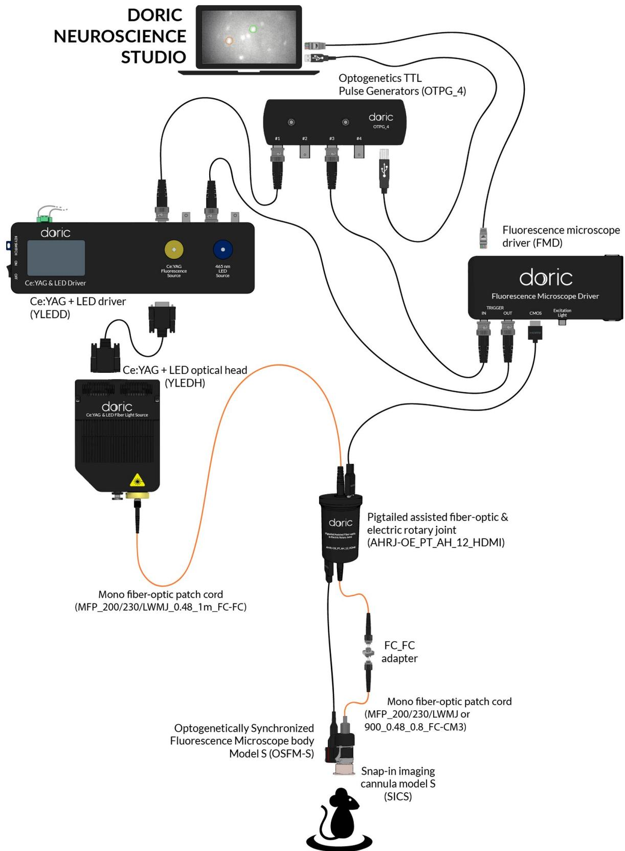
*Optogenetically Synchronized Microscopy System for Surface Imaging of GCaMP6 + NpHR3.0*
