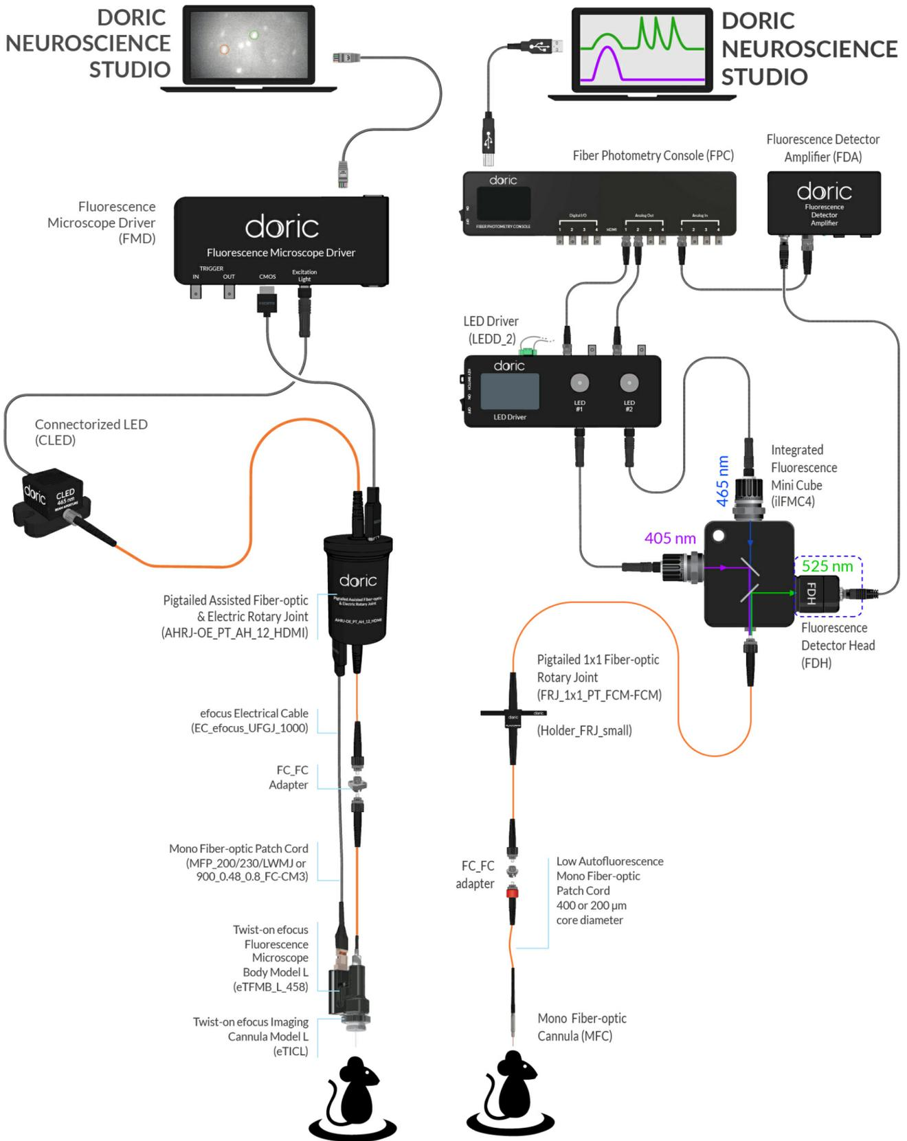
**(Left)** Miniaturized Fluorescence Microscopy System used for calcium imaging with GCaMP6. **(Right)** Fiber Photometry System with a 4 port Integrated Fluorescence Mini Cube and a Fiber Photometry Console.
