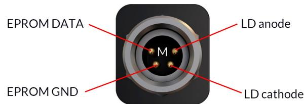
Connectorized Laser Diode Module male pinout
