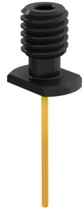
*Opto-fluid Cannula with interchangeable injectors*
