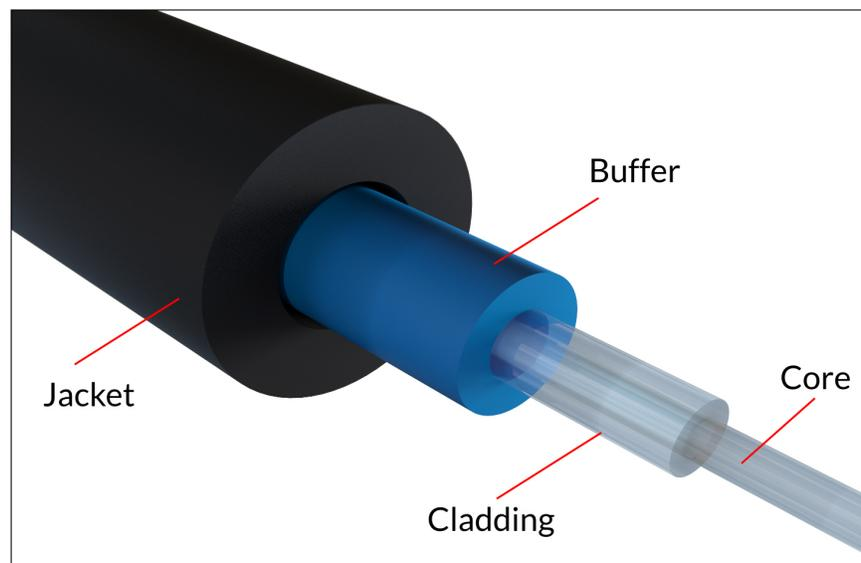
The *core* and the *cladding* are two layers that make up the lightguide. However, the light travels inside the core of the fiber-optic, barely or not inside the cladding. For this reason, interconnected fiber-optics should have the same core diameter. Different cladding diameters have no influence on the coupling efficiency.
