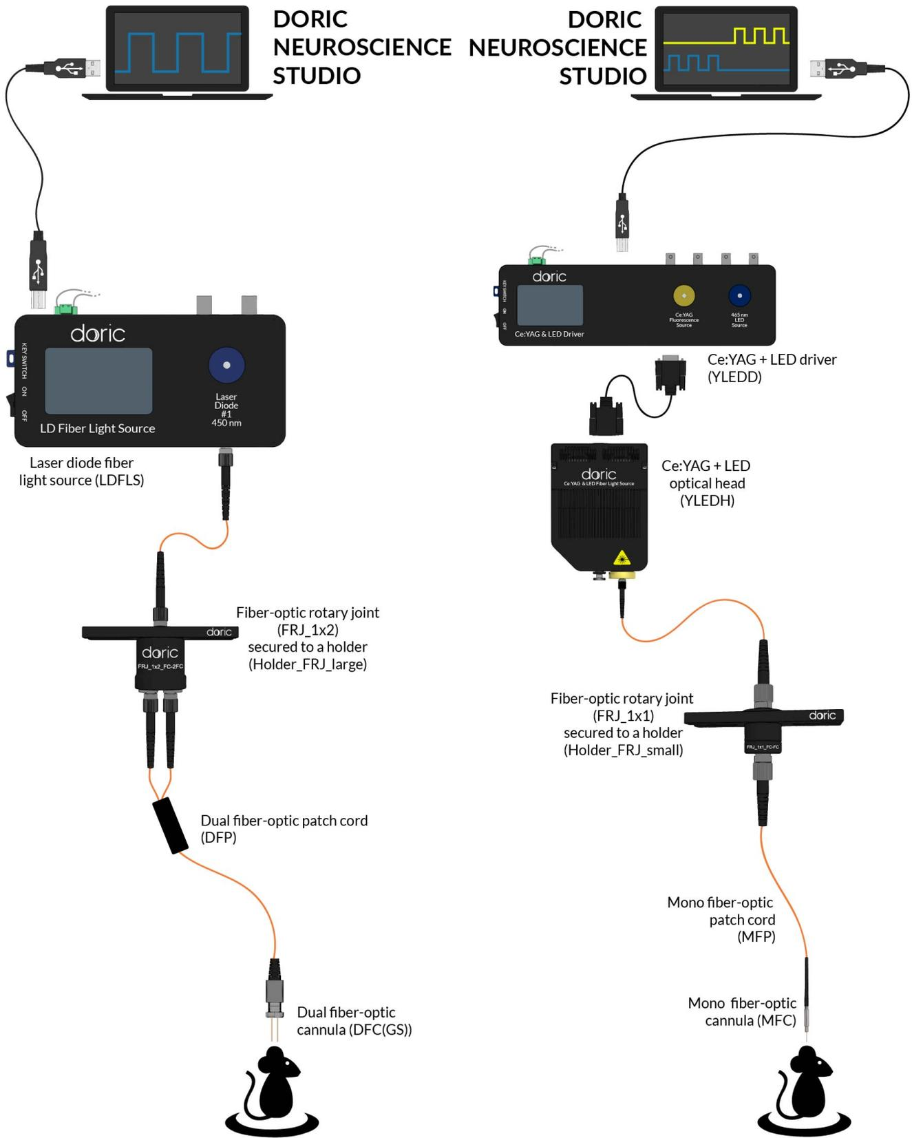
**(Left)** Dual optogenetic stimulation with a Laser Diode Fiber Light Source. **(Right)** 2-color optogenetic stimulation with a Ce:YAG + LED Fiber Light Source.
