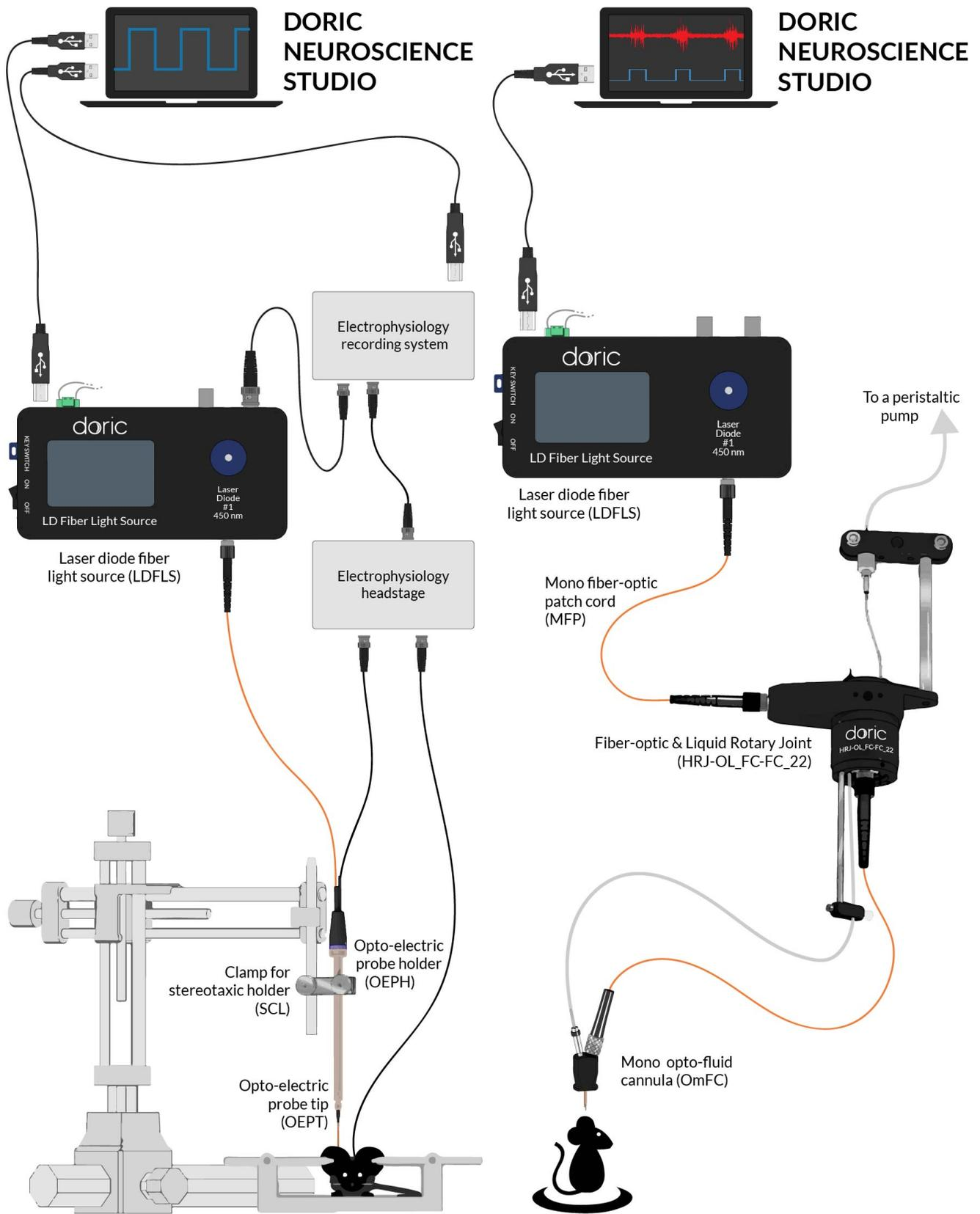
**(Left)** Optogenetic stimulation and electrophysiology recordings with an Opto-electric Probe Tip. **(Right)** Optogenetic stimulation and fluid delivery with a Mono Opto-fluid Cannula.
